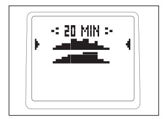
The workout time and a profile of the resistance levels for the workout will appear in the display.
