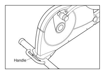
To unfold the elliptical exerciser, hold the handle, press the latch button, and lower the frame to the floor.
