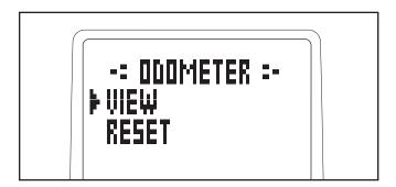
The total distance (in total number of revolutions) that the elliptical exerciser has been pedaled will appear in the upper display. The total number of hours the elliptical exerciser has been operated will appear in the lower display.
