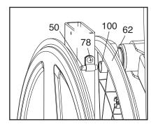
Reed Switch slightly closer to or away from the Magnet, and then retighten the Screw. Rock the Pulley Disc forward and backward just enough that the Magnet passes the Reed Switch repeatedly. Adjust the Screw until the console displays correct feedback. When the Reed Switch is correctly adjusted, reattach the shields. Note: If you have questions as to which screw should be in which hole, see EXPLODED DRAWING B on page 31 and the PART LIST on page 28.
